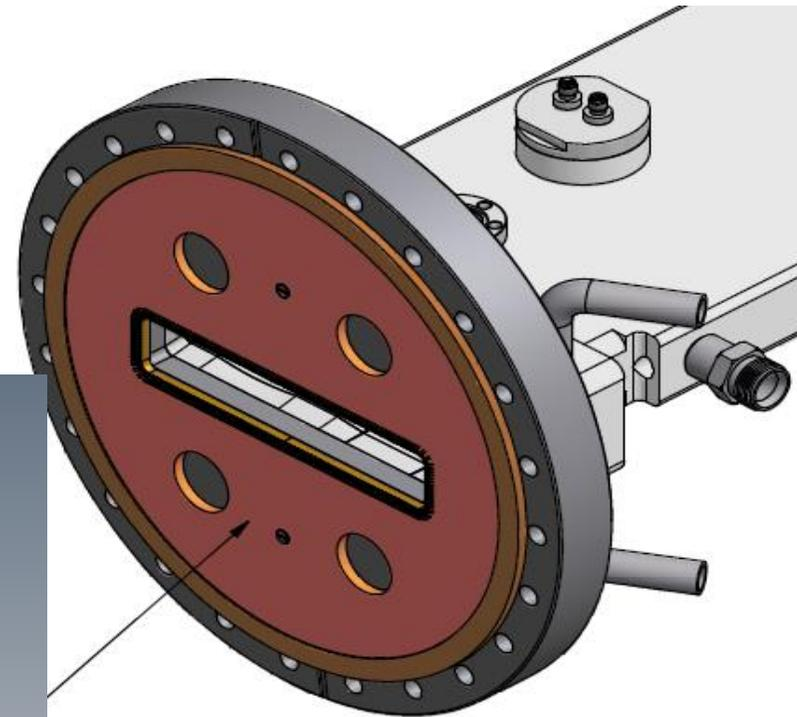
*Be-Cu RF Finger strip brazed onto Cu RF insert, to bridge the flange gap, on the vacuum side of the vacuum gasket.*
