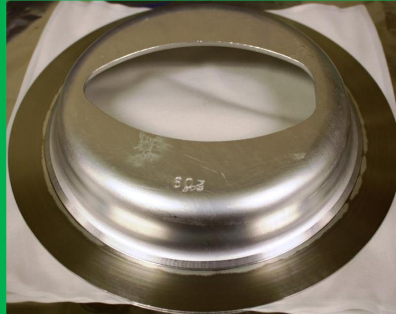
Friction bonded pans enable transitions between aluminum to stainless steel bellows
