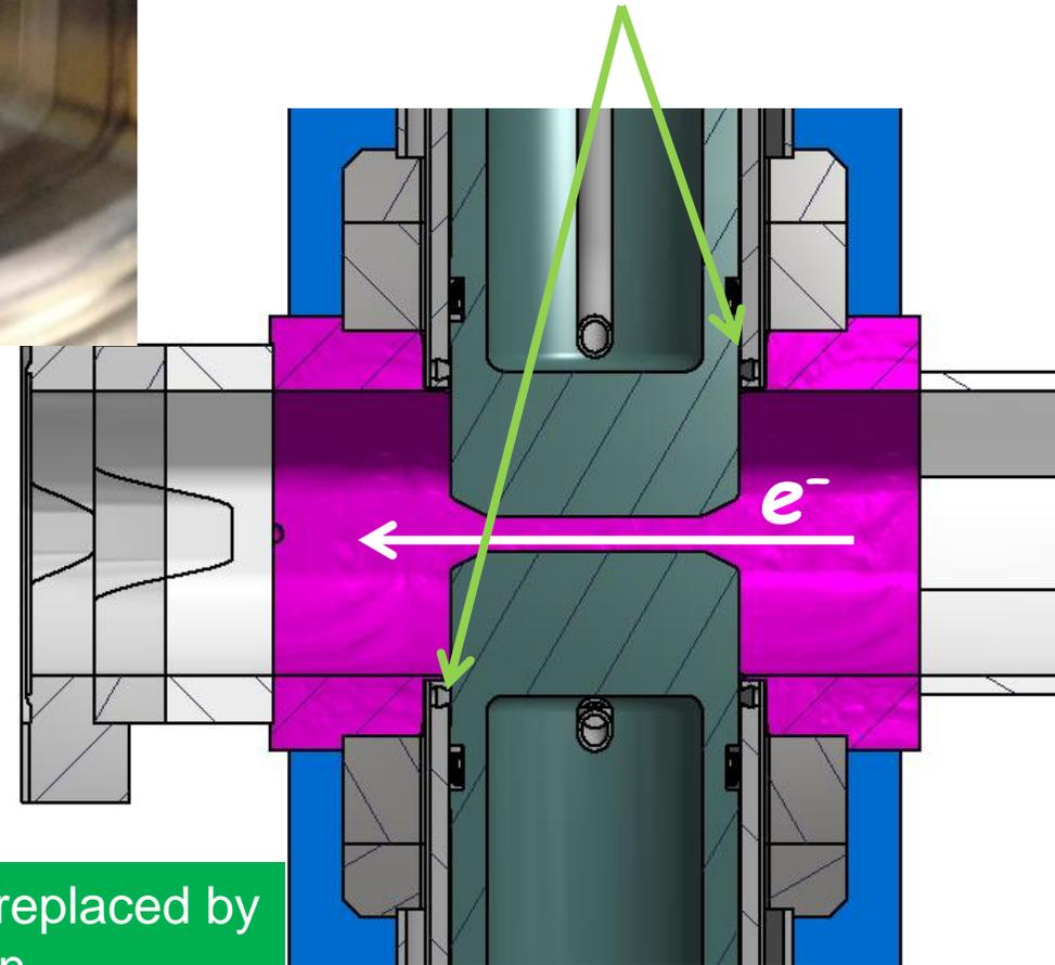
High resistive stainless coil springs were replaced by BeCu finger contact in an improved design
