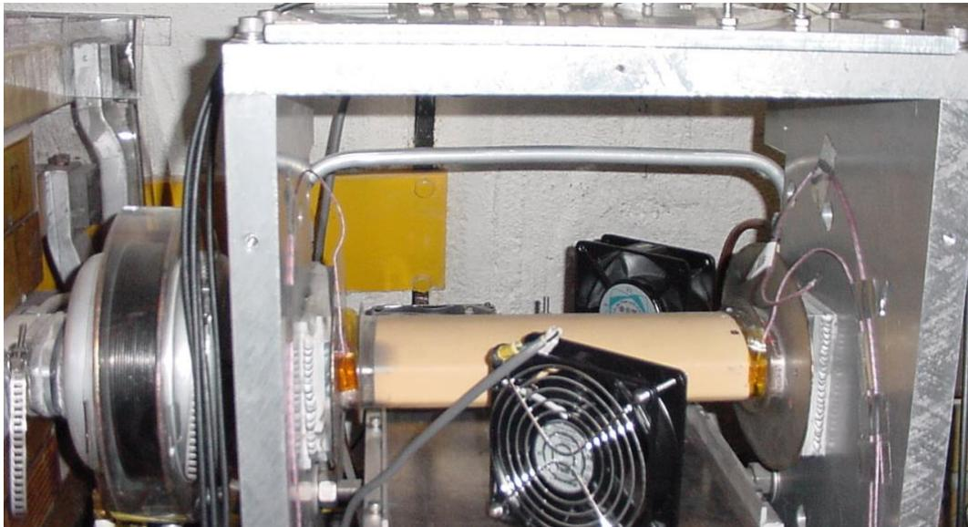
*A CESR ceramic pipe mounted on strong-back frame, with flexible ends*
