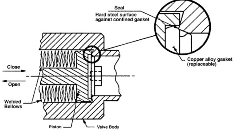
**Figure 1-1 Sealing Principle**
