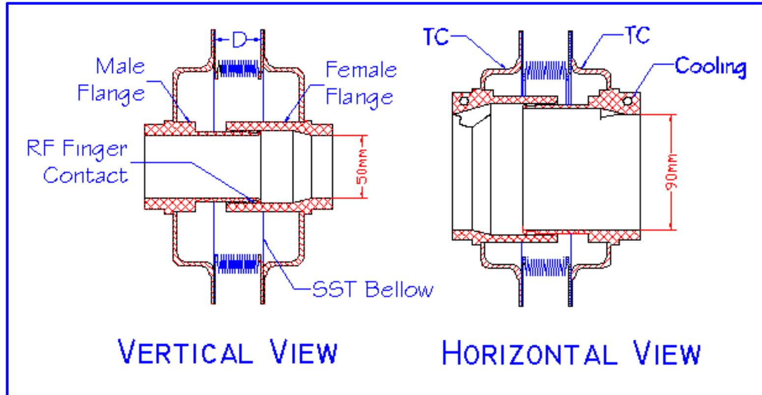
In storage rings (or accelerators with intense short bunched beams), bellows **MUST** be shielded from the beam. Otherwise, wake-field will be excited in the cavities to:
